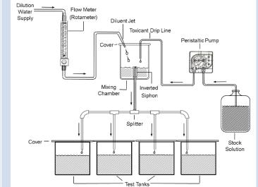
Maintain stable water quality and test concentrations (Diagram courtesy of EAG)
